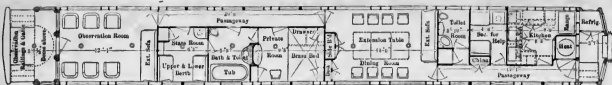
Fig. 2—Floor Plan of Private Car, Exhibit of F. M. Hicks &amp; Co.
